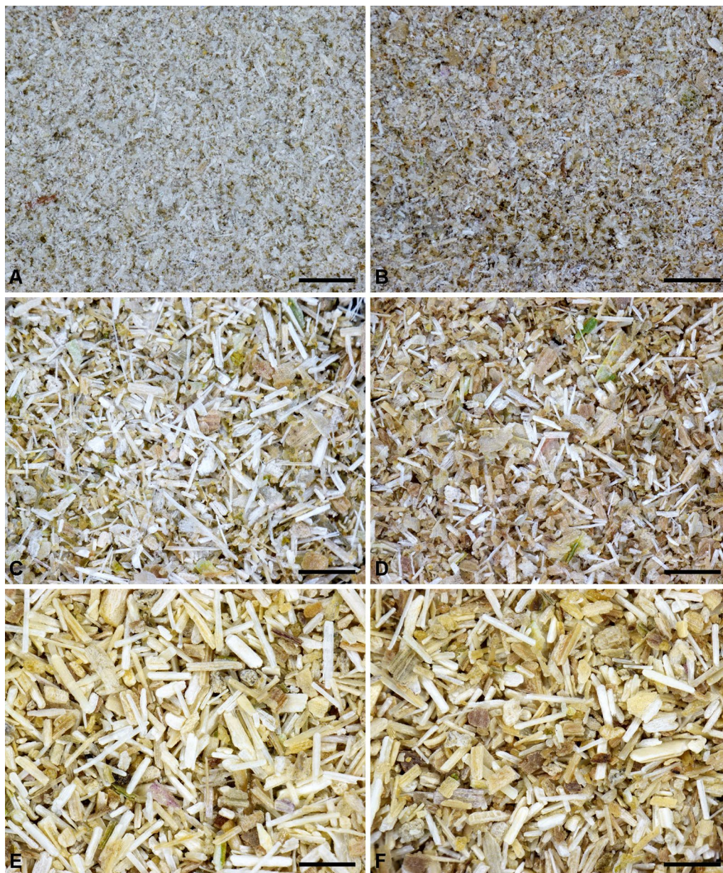
Fig. 2 Optical observation of fractions of maize shoot powder: a Mf+, b Mf-, c Mm+, d Mm-, e Mc+, f Mc- (the bar scale represents 500 \mu\text{m} )
