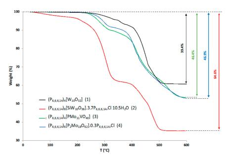
**Figure 2.** TGA curves recorded for compounds 1–4 under O<sub>2</sub> flow; heating rate of 5 °C/min.
