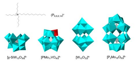
**Figure 1.** Representation of the cation and the POMs used in this study.  $MO_6$  octahedra (M = Mo or W) are given in blue, grey tetrahedra correspond to  $SiO_4$  or  $PO_4$  central tetrahedra and  $VO_6$  octahedron in the  $POM \left[PMo_{11}VO_{40}\right]^{4-}$  is highlighted in red.
