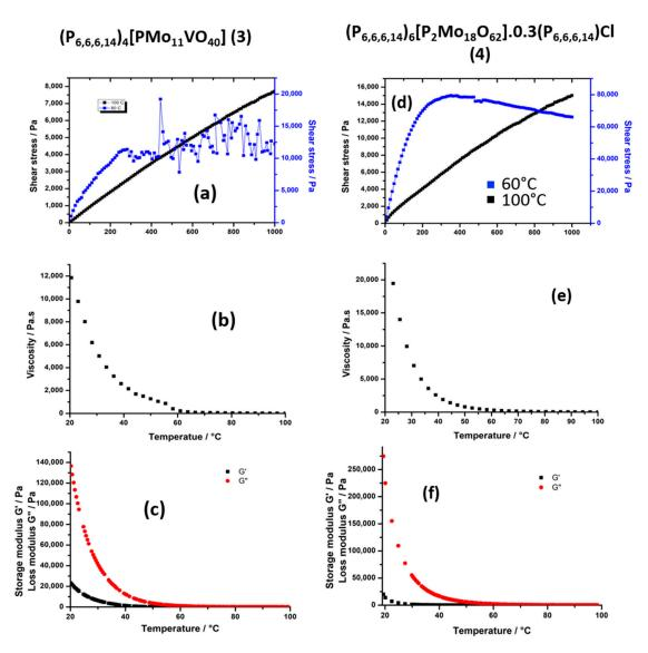
**Figure 6.** Flow curves  $\tau = f(\dot{\gamma})$  measured at 80 and 100 °C for **3** (a) an 60 and 100 °C for **4** (d); Viscosity variation as a function of the temperature between 20 °C and 100 °C ( $\dot{\gamma} = 10 \text{ s}^{-1}$ ) for **3** (b) and **4** (e); Temperature dependence of G' (black dots) and G" (red dots) with 20% strain and f = 1 Hz for **3** (c) and **4** (f).
