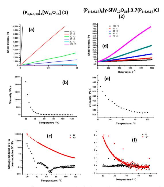
**Figure 5.** Flow curves  $\tau = f(\gamma)$  measured between 20 and 100 °C for **1** (a) and for **2** (d); Viscosity variation as a function of the temperature between 20 °C and 100 °C ( $\gamma = 10 \text{ s}^{-1}$ ) for **1** (b) and **2** (e); Temperature dependence of G' (black dots) and G" (red dots) with 20% strain and f = 1 Hz for **1** (c), and **2** (f).
