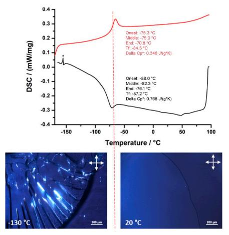
**Figure 4.** DSC traces in the heating (red) and the cooling (black) modes for compound **2**. Images taken at -130 °C and +20 °C by Polarized Optical Microscopy (\* = artefact).
