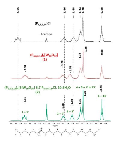
**Figure 3.** <sup>1</sup>H NMR spectra comparing  $(P_{6,6,6,14})_4[W_{10}O_{32}]$  (1),  $(P_{6,6,6,14})_8[SiW_{10}O_{36}] \cdot 3.7P_{6,6,6,14}Cl$  10.5H<sub>2</sub>O (2) and  $(P_{6,6,6,14})Cl$  in acetone- $d_6$ .
