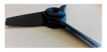
**FIGURE 2** A310 impeller used in this study coated with black paint to minimize laser refraction [Color figure can be viewed at wileyonlinelibrary.com]
