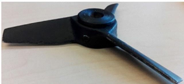
**FIGURE 2** A310 impeller used in this study coated with black paint to minimize laser refraction [Color figure can be viewed at [wileyonlinelibrary.com](http://wileyonlinelibrary.com)]
