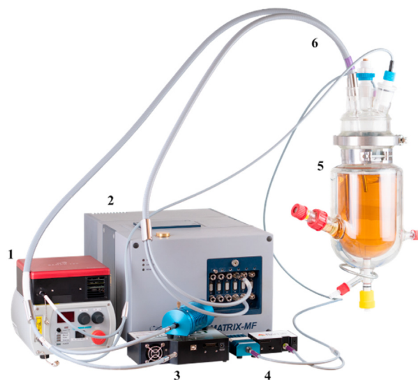
Fig. 1. Scheme of multispectral fiber system (figure courtesy of Art Photonics GmbH, Germany [26]). Raman system (1); FTIR absorption system (2); NIR reflection system (3); fluorescence detector (4); chemical reactor (5); and fiber optic probes (6).
