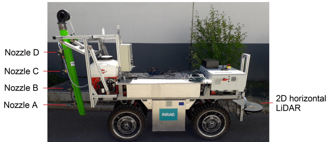
Fig. 3. Experimental robot carrying a vertical air-assisted sprayer with four independent nozzles placed at different working heights
