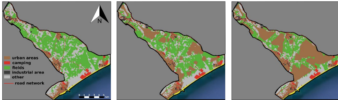
Figure 1: Illustration of urban expansion (from left to right) in a river delta flowing into the Mediterranean Sea, as modelled with a cellular automaton using the NetLogo® platform. The urban areas (brown areas) are constrained by the distance to the road network (red lines) and the distance to the sea. The background image is taken from Google Maps® and land uses derive from a study on the Lower Orb river fluvial plain by Saint-Geours et al. (2015).
