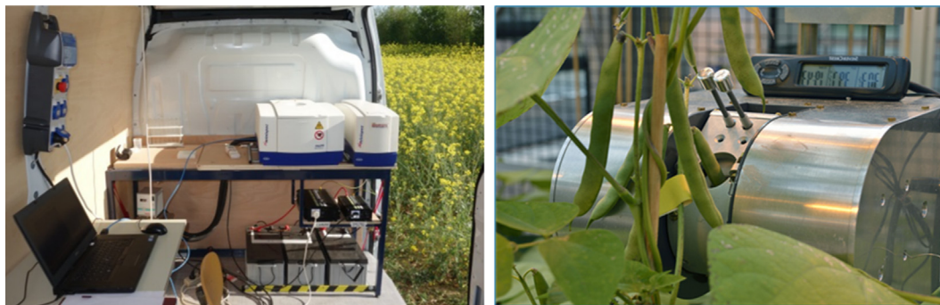
Fig. 1. Left -mobile TD-NMR lab with conventional spectrometer next to a field of oilseed rape. Adapted from Publication [38], Copyright (2017), with permission from Springer Nature; Right - small scale C-shaped magnet measuring water dynamics of growing bean pod in a greenhouse [53].
