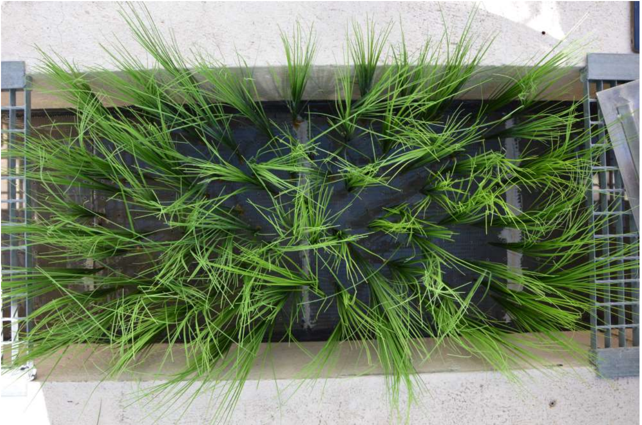
184 Figure 3: Picture of the vegetated area ( Isolepis sp.) in the experimental channel (36 plants per 185 concrete panel on two panels).
