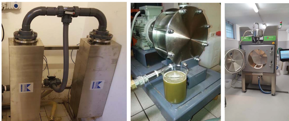
Fig. 13 Continuous ultrasound – cavitation reactor – pilot scale microwave extractor.
