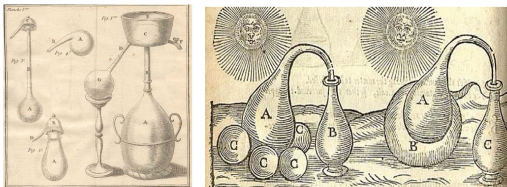
Fig. 1 Innovative alembics by Macquer (1756) 2 and French (1651). 3
