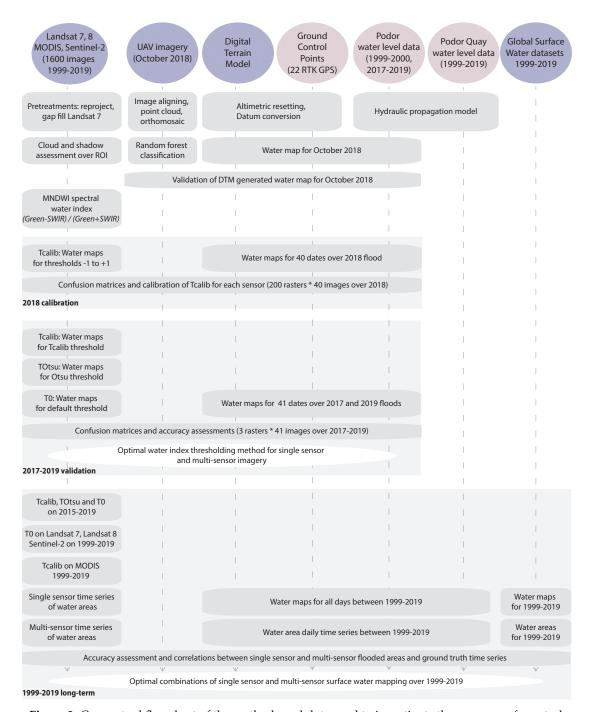
**Figure 2.** Conceptual flowchart of the methods and data used to investigate the accuracy of spectral water index thresholding methods and optimal combinations of single sensor and multi-sensor imagery.
