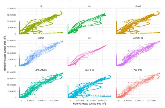
**Figure 13.** Scatterplot of daily interpolated remotely sensed flooded areas and ground truth data from each sensor and multi-sensor combinations (1999–2019).
