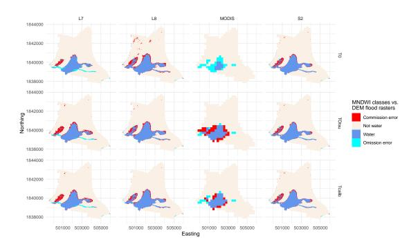
**Figure 8.** MNDWI classifications from four sensors based on three thresholding methods during a low flood, September 2017.
