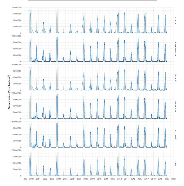
**Figure 14.** Comparison of multi-sensor remotely sensed flooded areas with the optimal MNDWI classification method and from Global Surface Water datasets (blue lines) against ground truth data (grey areas) (1999–2019).
