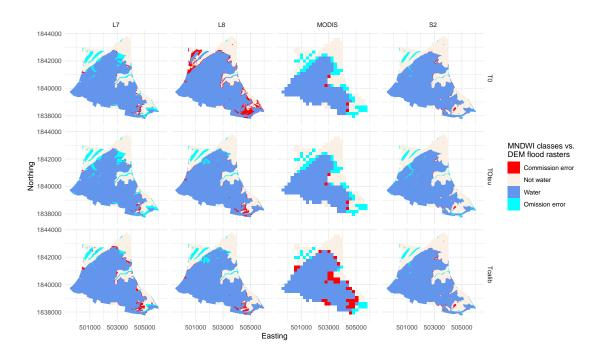
**Figure 9.** MNDWI classifications from four sensors based on three thresholding methods during a high flood, October 2018.
