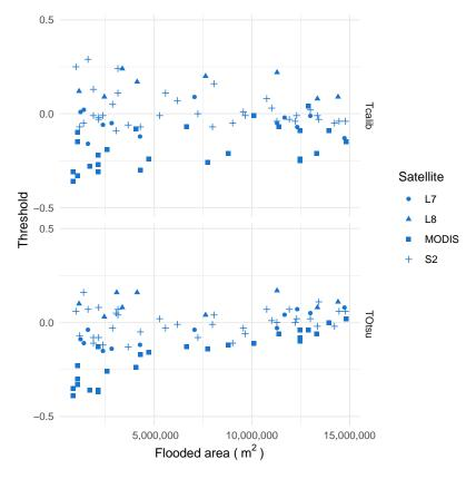
**Figure 5.** Comparison of optimal threshold based on the Otsu algorithm (TOtsu) and on calibration against field data (Tcalib) for Landsat 7, Landsat 8, MODIS and Sentinel-2 as a function of the flooded area.
