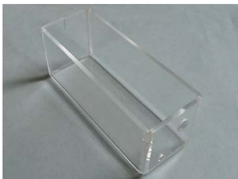
Figure 1. Custom made transparent Plexiglass® growth monitoring chamber
