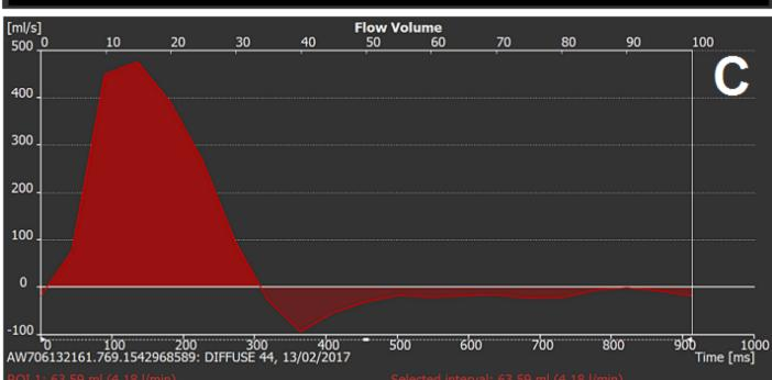
Forward flow volume: 79.48 ml 5.22 l/min Backward flow volume: 15.89 ml 1.04 l/min
