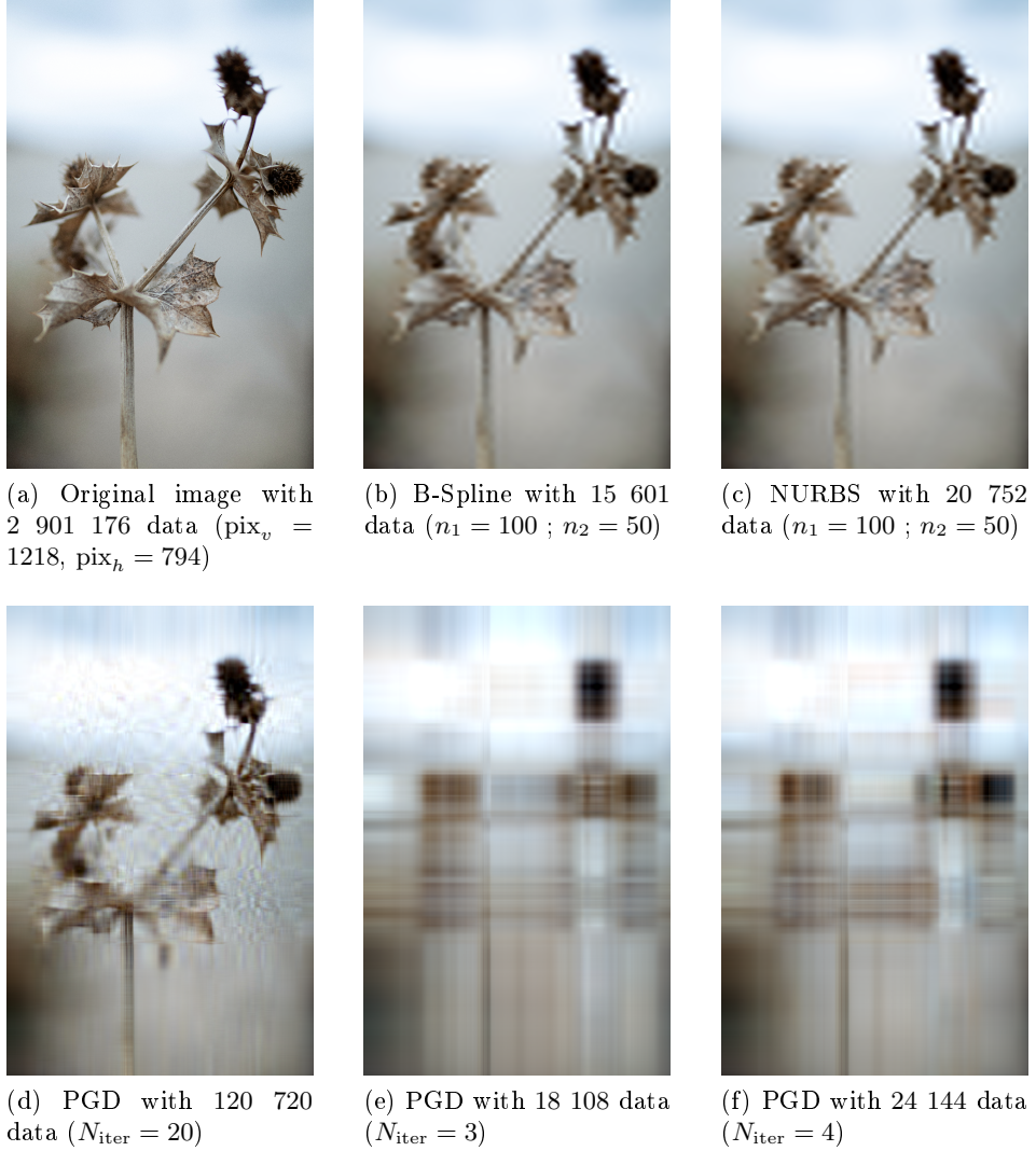
Figure 10: Image reduction: comparison between PGD [1], NURBS and B-Spline results for a maximum relative error equal to 0.65.
