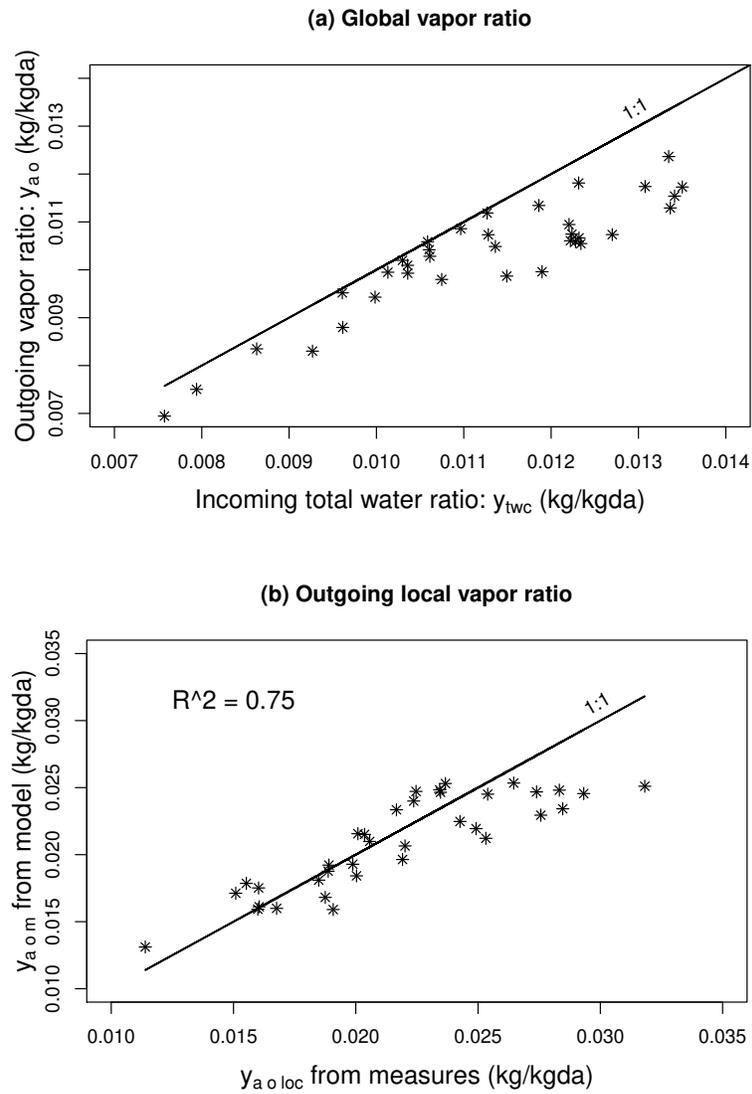
Figure 5: (a) Outgoing vapor ratio  $y_a$ , as a function of incoming total water ratio in air and (b) modelled vapor ratio  $y_m$  versus measured one  $y_{a,o,loc}$  (b)
