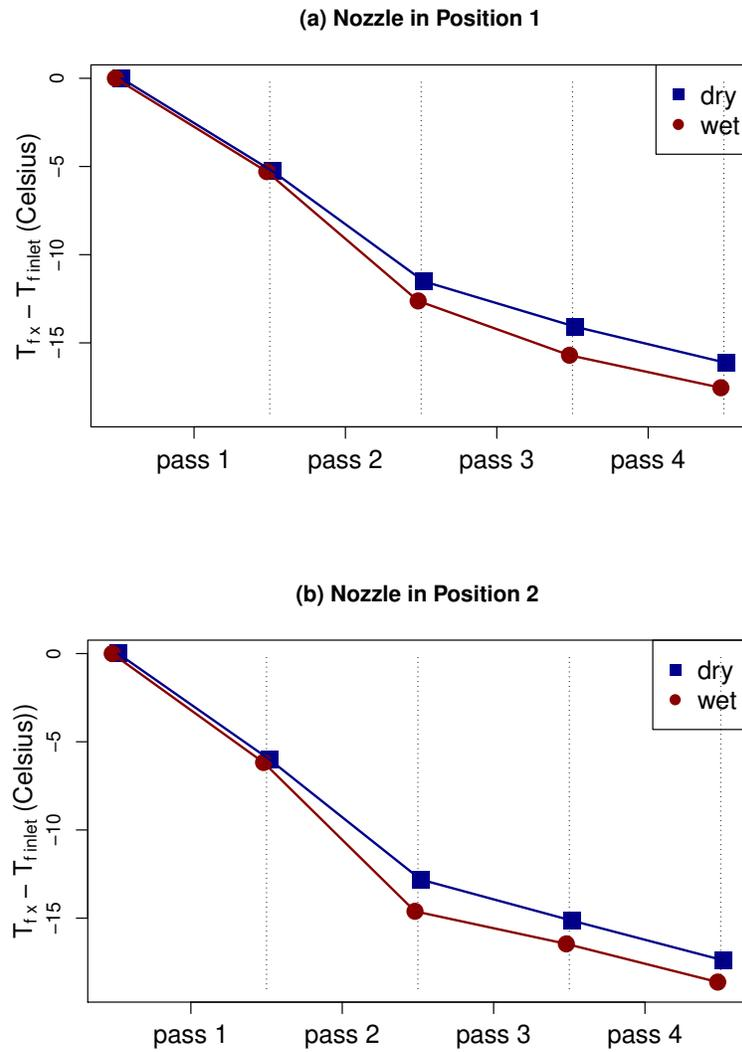
Figure 2: Fluid temperature profiles along the heat exchanger without and with spraying for nozzle position 1 (a) and nozzle position 2 (b) -  $T_{f,i} = 70^\circ$ ,  $m_s = 1$  L/h,  $m_a = 0.2$  kg/s,  $m_f = 0.078$  kg/s,  $T_{a,i} = 27^\circ\text{C}$ ,  $HR_{a,i} = 37\%$
