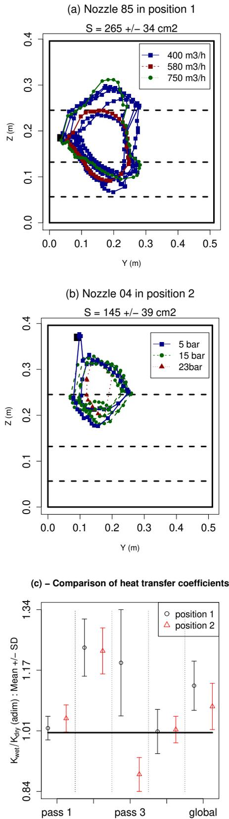
Figure 4: Impacted area for position 1 (a) and 2 (b) and (c) related changes in heat transfer coefficient for each exchanger pass
