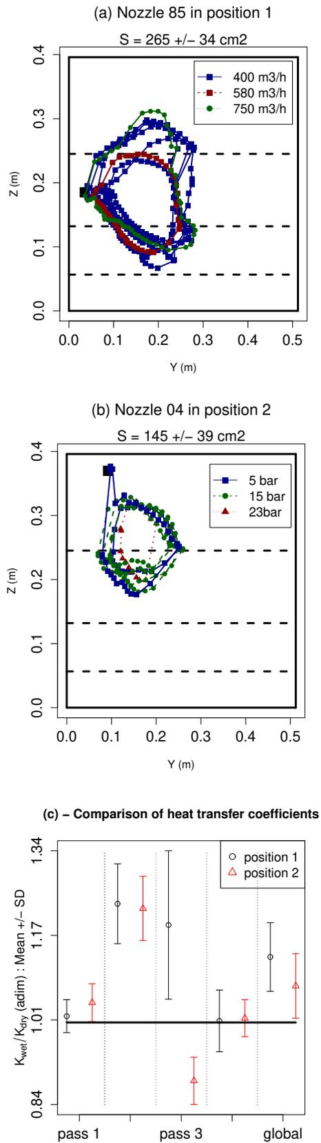
Figure 4: Impacted area for position 1 (a) and 2 (b) and (c) related changes in heat transfer coefficient for each exchanger pass
