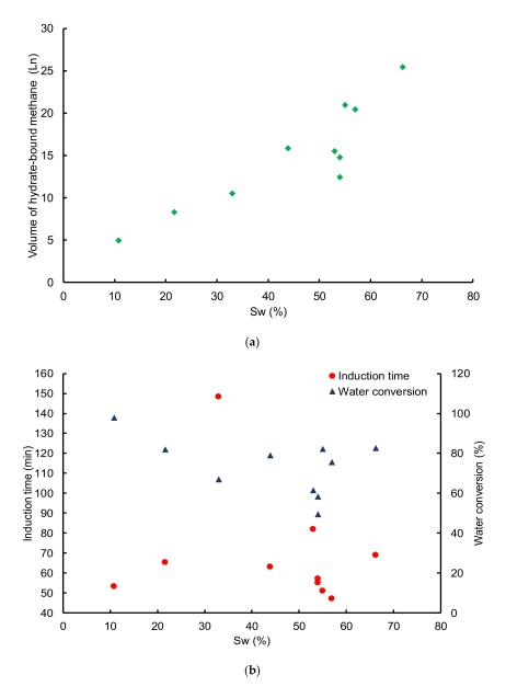
**Figure 8.** (a) Volume of hydrate-bound methane as a function of water saturation; (b) Induction time and water conversion as a function of water saturation. The experiments were carried out with a non-sieved sand sample and a gas flowrate around  $58 \text{ mLn}\cdot\text{min}^{-1}$ .
