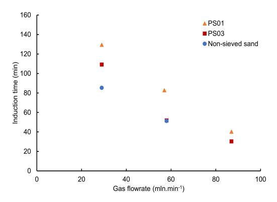
Figure 11. Induction time as a function of gas flowrate for a water saturation around 53%.
