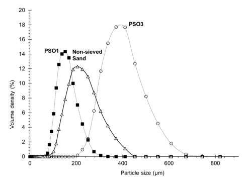
**Figure 1.** Experimental particle size distribution of calibrated Fontainebleau sand by diffractometer analysis: ( $\Delta$ ) non-sieved sand; ( $\blacksquare$ ) class PS01 particle; (•) class PS03 particle. Lines are used only to guide the eye.
