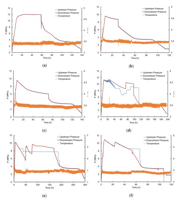
**Figure 7.** Upstream and downstream pressure and temperature profiles for experiments with non-sieved sand, a gas flowrate around 58 mLn·min<sup>-1</sup> and different water saturations  $S_w$ : (a)  $S_w = 10.8\%$ ; (b)  $S_w = 21.6\%$ ; (c)  $S_w = 33\%$ ; (d)  $S_w = 44\%$ ; (e)  $S_w = 55\%$ ; (f)  $S_w = 66.3\%$ .
