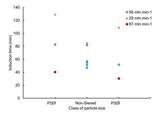
Figure 9. Induction time as a function of particle size for a water saturation around 53%.
