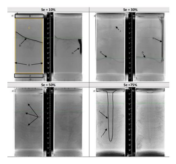
**Figure 5.** Orthogonal views of tomographic images of the sandy core for different water saturations (1) 10%, (2) 30%, (3) 50%, (4) 75%: (**a**) and (**b**) are orthogonal orientations. (A, E, G) Aluminum walls, (B, F) porous bauxite stones, (D) waterfront, (H) Thermometer hole, (I) high-water-content region, (J) cryogenic fracturing.
