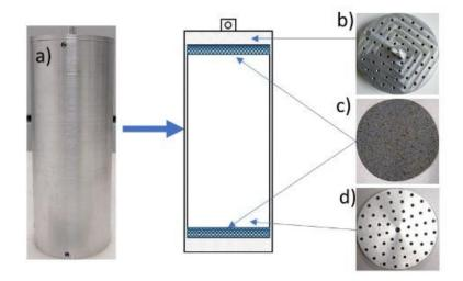
**Figure 4.** Photos and description of the interior of the aluminum cell: (**a**) aluminum body, (**c**) porous bauxite stones, (**b**,**d**) perforated aluminum lids.
