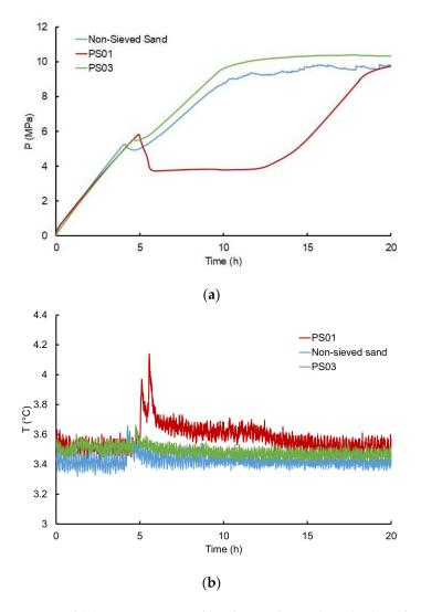
**Figure 10.** (a) Pressure and (b) temperature profiles during the methane hydrate formation step at around 53% water saturation and a gas flowrate of 29 mLn·min<sup>-1</sup> with different classes of particle sizes.
