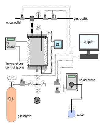
**Figure 2.** Schematic diagram of the experimental apparatus. (DL) Data logger, (P) Pressure regulator, (F) Mass flow regulator, (Pt) Pressure transducer, (T) Thermocouple, (TR) thermal regulator, (VP) Vacuum Pump,(•) high-pressure filter for gas-liquid separator, (**I**) high pressure 0.5 µm filter.
