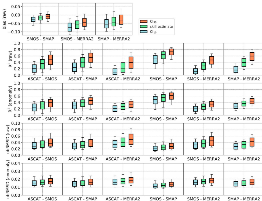
Fig. A.9. Spatial summary statistics of biases [ m^3m^{-3} ], ubRMSDs [ m^3m^{-3} ], and coefficients of determination [-] and their 10% and 90% confidence limits, respectively, for raw soil moisture estimates and soil moisture anomalies of ASCAT, SMOS, SMAP and MERRA-2. Boxes represent the (spatial) median and inter-quartile-range and whiskers represent the 5 and 95 percentiles.
