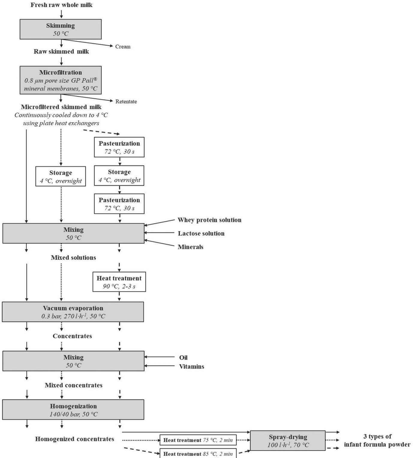
**Figure 1.** Semi-industrial process flow diagram for production of 3 types of infant formula powders. Solid arrow = T- (no heat treatment), round dot arrow = T+ (moderate heat treatment), hyphen arrow = T+++ (intense heat treatments).
