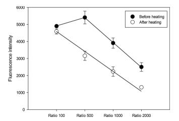
Fig. 3. Fluorescence intensity of FG-FS at different grafting FS / fluorophore ratios, in native conditions (filled circles) and after heating (165  $^{\circ}\text{C}$  for 8 min; empty circles). All measurements are done in triplicate, some standard deviations are weak and so not visible.
