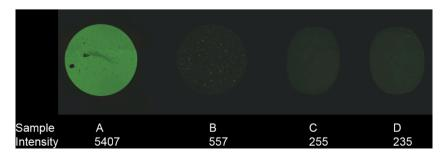
Fig. 11. Evolution of fluorescence of FG-FS (ratio 500) material along the process. A: native FG-FS particles. B: FG-FS particles mixed (10 % w/w) with FS particles. C and D: compound and filament FG-FS material (fluorescence measurement with LED light power: 100 %, exposure time: 400 ms).
