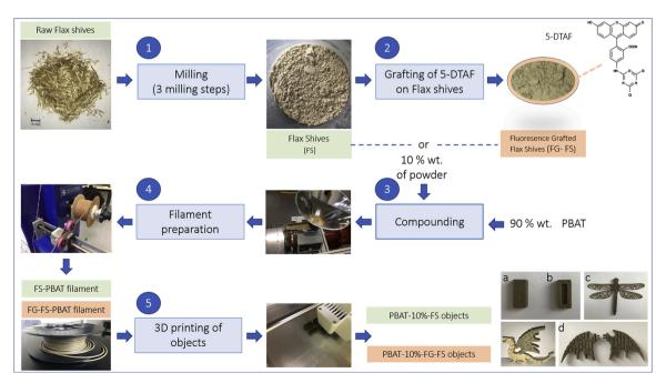
Fig. 2. Overview of the steps to produce fluorescent 3D printed composites from flax shives.
