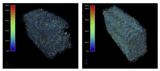
Fig. 9. Volumic distribution of particles in FS (A) and FG-FS (B) samples according to their size.
