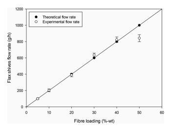
Fig. 7. Comparison between experimental and theoretical FS flow rate during the compounding dosing step.
