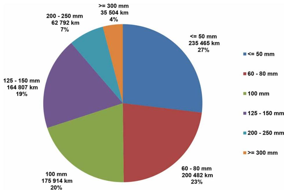
Figure 6 | Spread of pipe length by diameter.
