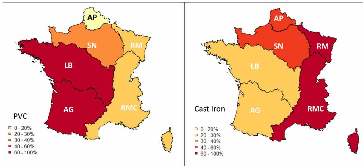
**Figure 8** | Proportions of PVC and cast iron pipes by WA.
