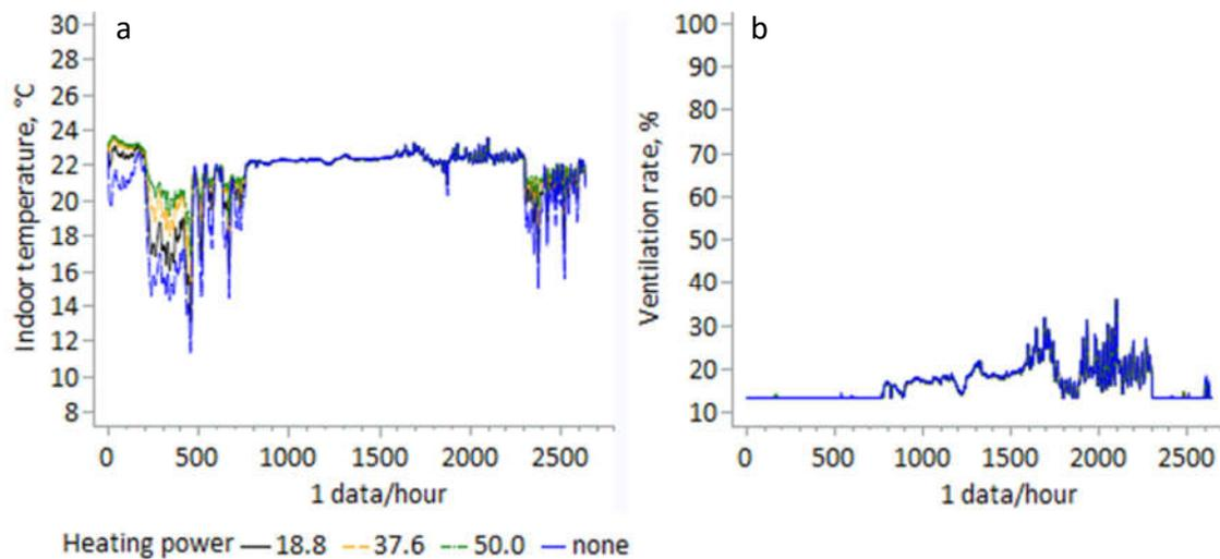
Figure 4. Effect<sup>1</sup> of the heating power capacity (W/pig) on the hourly indoor temperature (a) and ventilation rate (b) all along the fattening period under the SW01 climate<sup>2</sup>
