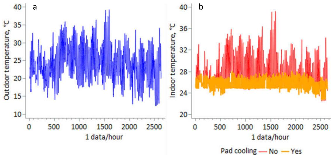
Figure 5. Hourly outdoor temperature under FR06 climate (a) and effect<sup>1</sup> of pad cooling on the hourly indoor temperature (b).
