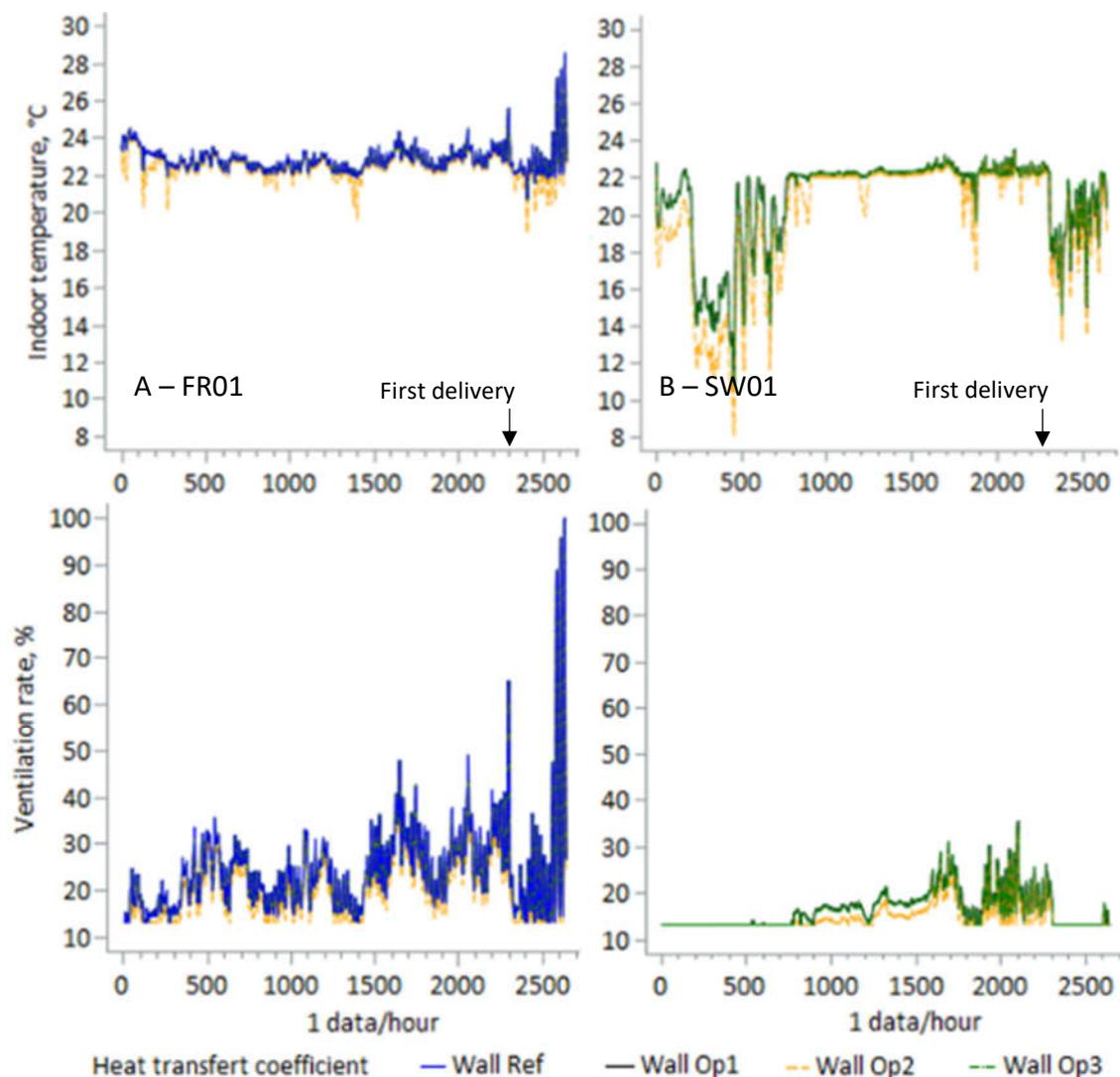
Figure 3. Effect of the heat transfer coefficient (HTC) of walls<sup>1</sup> on the hourly indoor temperature (a, b) and the ventilation rate (A, B) all along the fattening period either under the FR01<sup>2</sup> (a, A) or the SW01<sup>3</sup> (b, B) climate.
