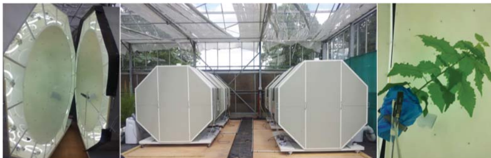
Fig. 1: Isotropic light illumination system. Going left to right: 1) the two hemispheres with their white circle neon lights and the sample attaching device, 2) the four modules used in this study placed in a greenhouse, 3) poplar plant fixed on the attaching device. Photograph courtesy of Richet N.
