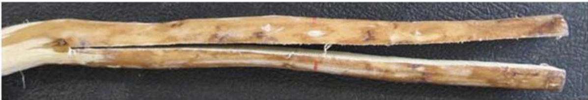
Fig. 1: Sample after the "Splitting" test has been performed. The opening is measured and used for the strain calculation along with diameter and cut length. This sample shows significant growth-strain as can be seen from the wide opening.
