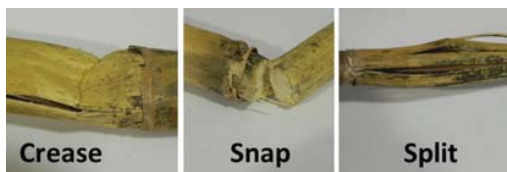
Fig. 1: The three modes of maize stalk failure.
