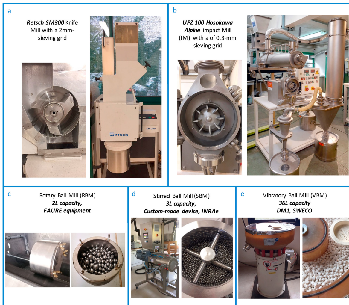
Fig. 1. Milling devices used: (a) knife mill, (b) impact mill (IM), (c) rotary ball mill (RBM), (d) stirred ball mill (SBM), and (e) vibratory ball mill (VBM).
