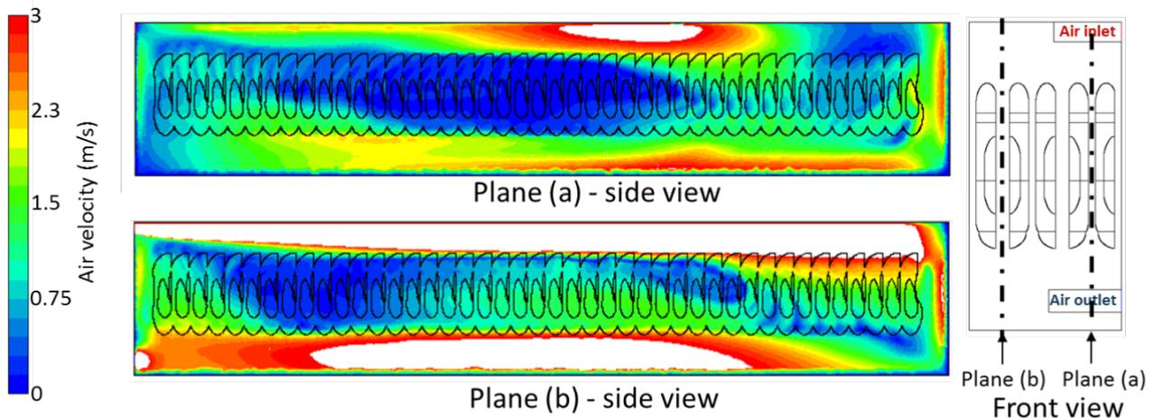
**Figure 7 : Velocity magnitude between half carcasses**
