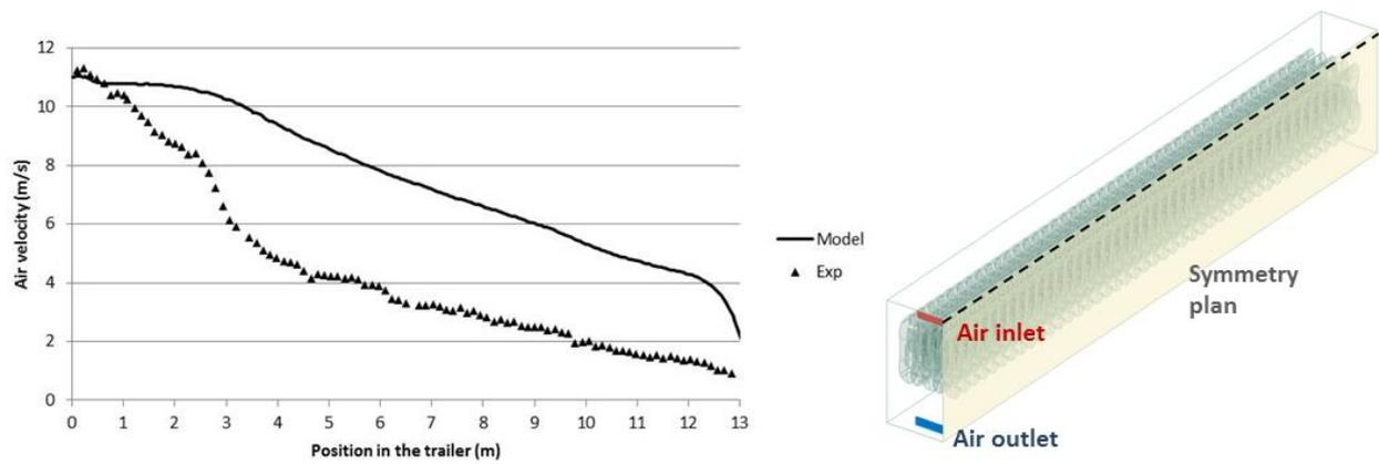
**Figure 6 : Velocity along the jet axis**
