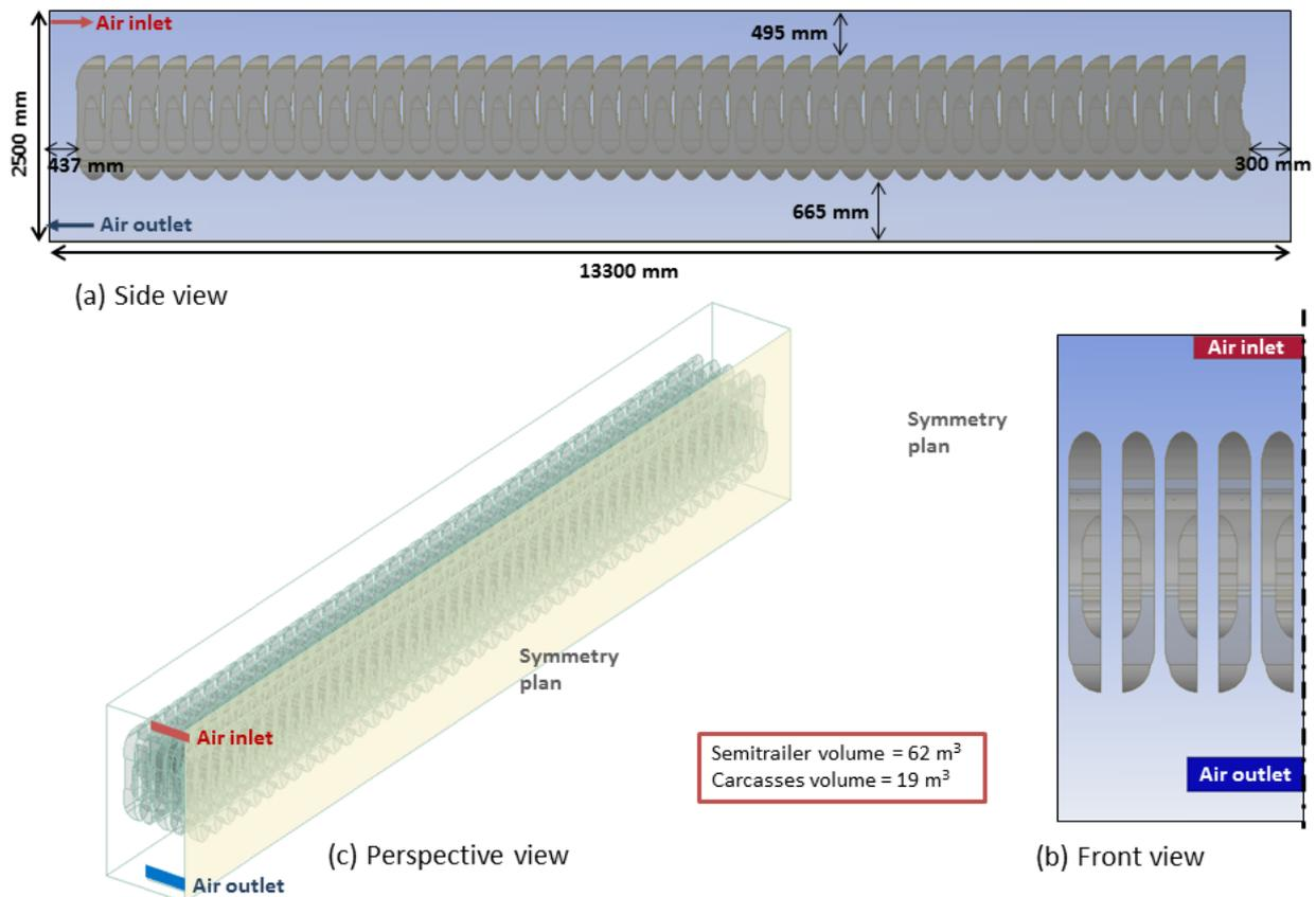
**Figure 1: Dimensions of the trailer (real scale)**
