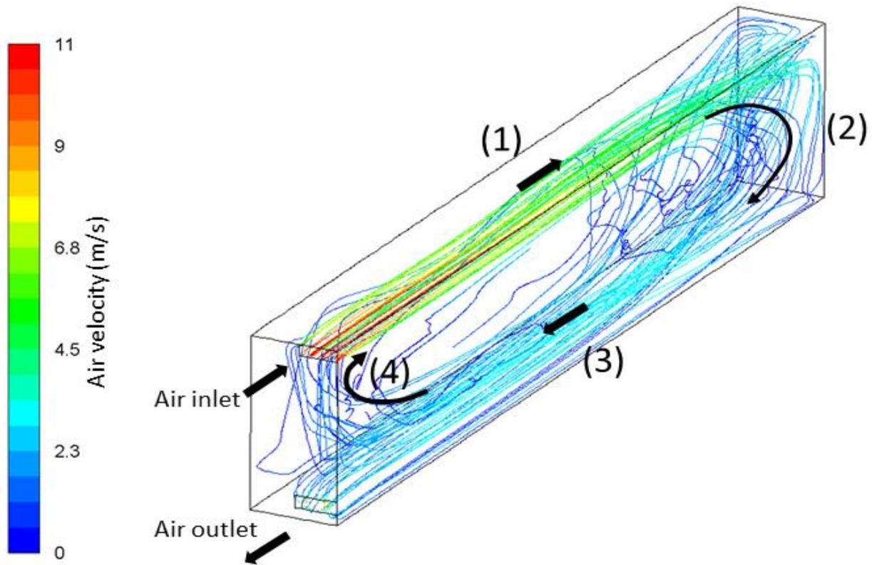
**Figure 4 : Stream lines issued from the inlet section**
