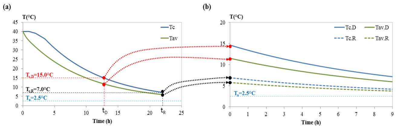
**Figure 3: Carcass core and average temperature changes during refrigeration: (a)-in a cold room of a slaughterhouse; and (b)-in a semi-trailer (Dotted lines show the corresponding temperatures of carcasses transferred from a cold room to a semitrailer)**
