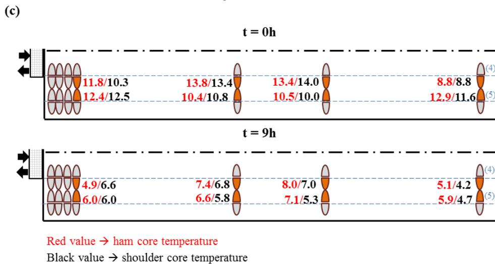
Figure 2: (a) - Product and air temperature changes during transport (9 h) of the carcass C3; (b) - Product surface temperature (c) - Product core temperature at the beginning (t=0) and at the end (t=9h) of transport
