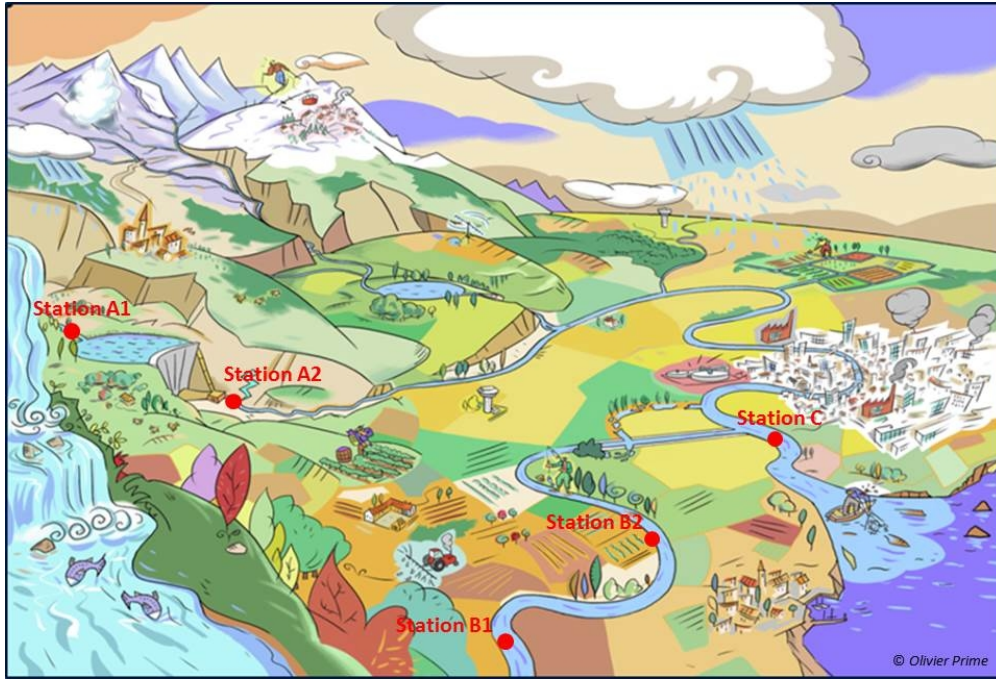
A catchment impacted by human activities: gauging stations A1 and B1 are uninfluenced, gauging stations A2, B2 and C are candidates for naturalization procedures (Source: INRAE)
