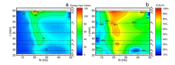
505 Fig. 14 Spectrum of total energy input and periodic contribution as a function of mixing rate and 506 radius
