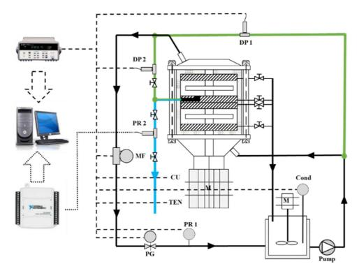
181 Fig. 2 Experimental set-up. Mean and instantaneous pressure measurements are illustrated by 182 green (differential pressure, DP1 and DP2) and blue (relative pressure, PR2) lines.
