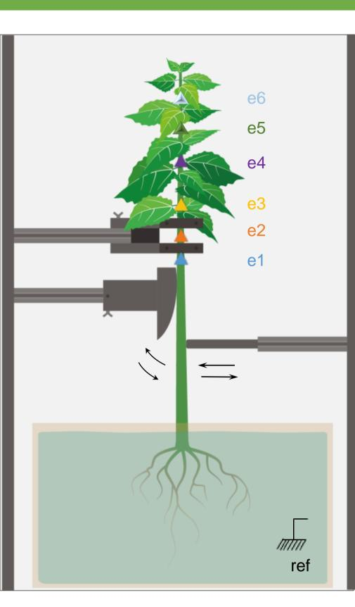
The speed and the magnitude of the bending stimulation were controlled by a motorized arm that pushed the stem against a plastic template, which had a constant radius of curvature. The setup was adjusted to apply a maximal peripheral longitudinal strain of the bark  $\varepsilon_{max}$  of around 2% (Coutand *et al.*, 2009). This method allowed applying the same strain level along 12 cm of the bent segment.
