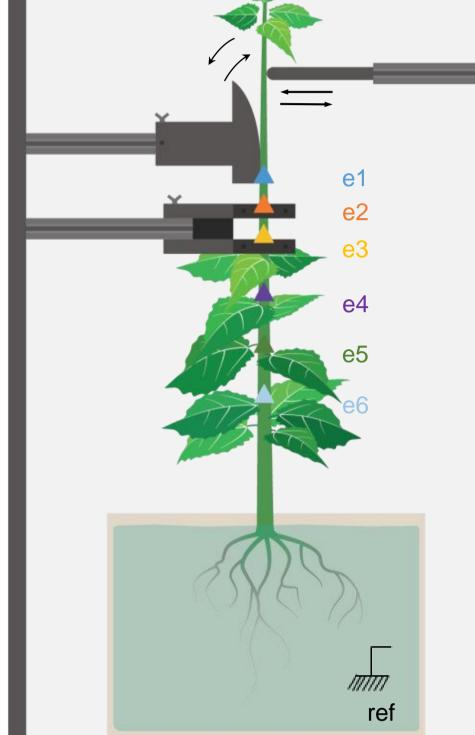
suspended in a nutrient solution. Six measuring electrodes are inserted in the immobile part of the stem and the reference electrode is placed in the solution. The electrical potential recorded is the difference between a measuring electrode and the reference electrode with respect to the ground. In contrast to intracellular measurements, extracellular measurements show potential changes downward for depolarization and upward for hyperpolarization.
