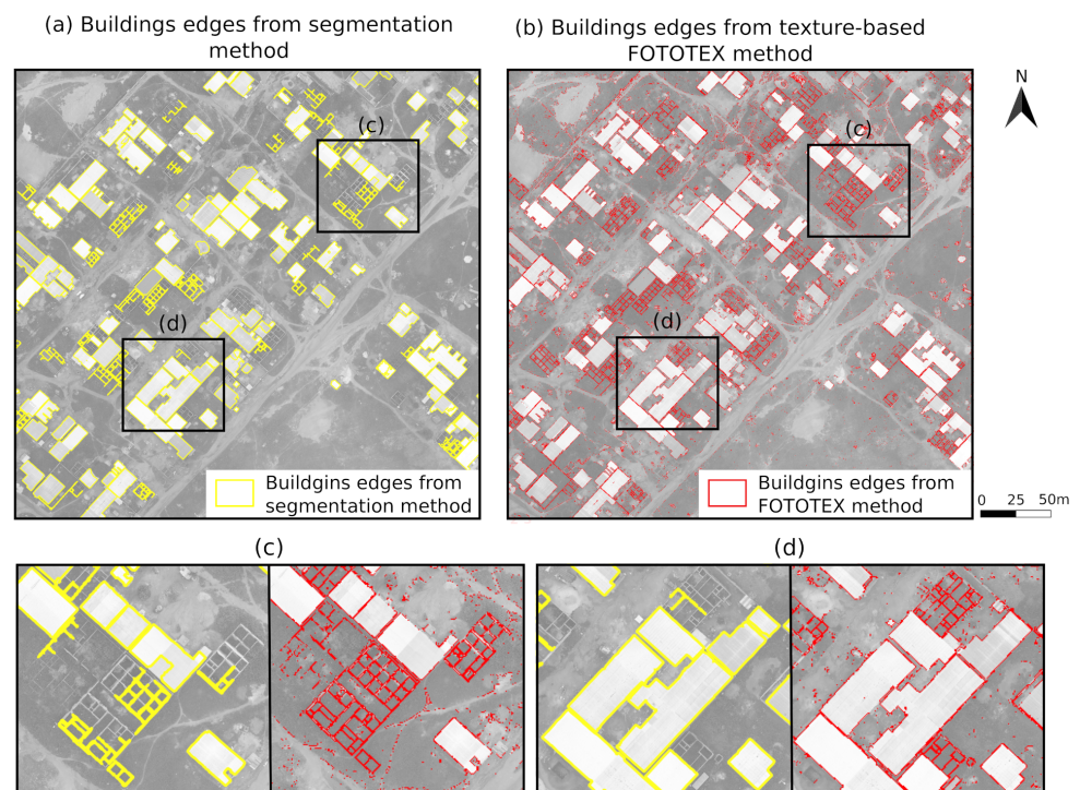
Figure 13. Extraction of buildings edges with (a) a segmentation method carried out with the Large Scale Generic Region Merging algorithm (Orfeo Toolbox) and (b) the FOTOTEX method implemented on the blue band of UAV image. (c,d) zooms on two different areas to compare detection by FOTOTEX and segmentation.
