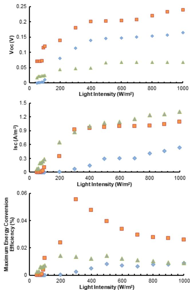
**Fig 7.** Performance parameter of DSSCs using Bx (◆), Bx-Zn (■), and Bx-Cu (▲) as sensitizer and KI-I<sub>2</sub> electrolyte system
