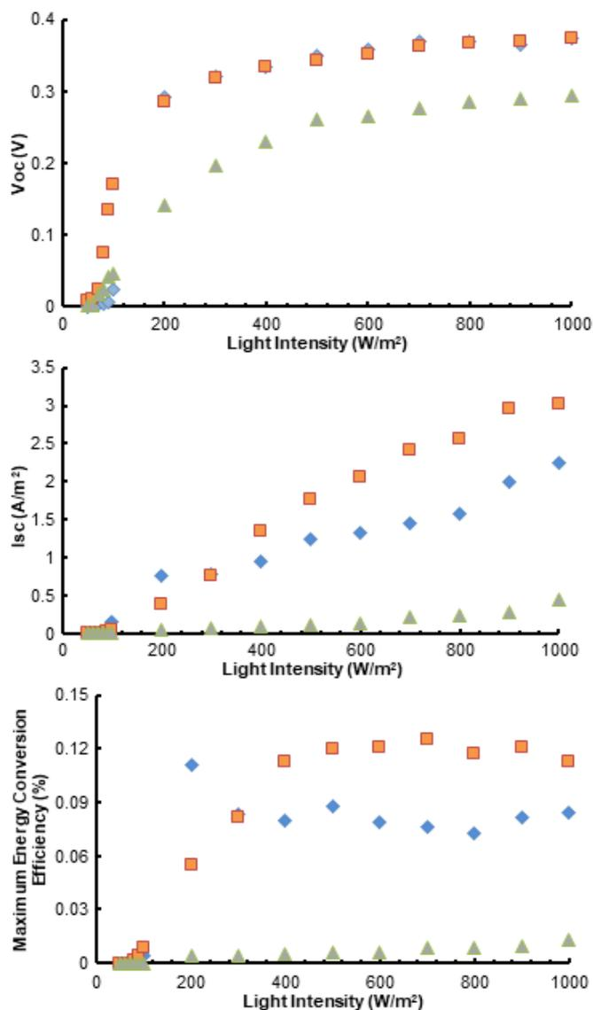
**Fig 8.** Performance parameters of DSSCs using Bx (◆), Bx-Zn (■), and Bx-Cu (▲) as sensitizer and KI-I<sub>2</sub> + MPII 0.4 M electrolyte system
