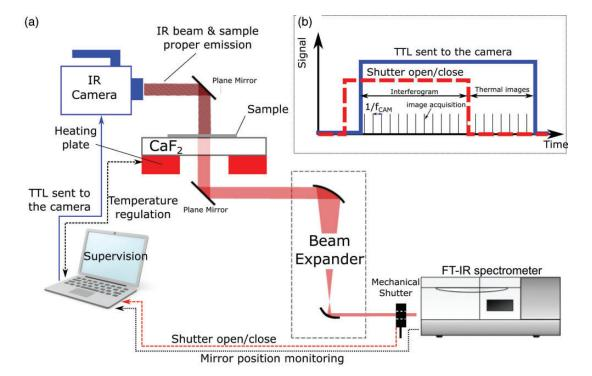
**Figure 1.** (a) Schematic of the fast thermospectroscopic imager. The IR camera can be either the InSB or SLS camera in this study. (b) Signal processing used to synchronize the instruments. IR: infrared; TTL: transistor-transistor logic;  $CaF_2$ : calcium fluoride.
