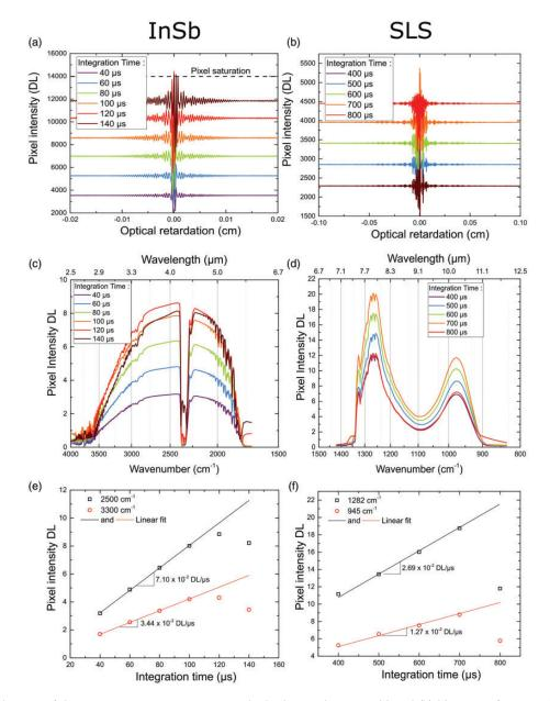
**Figure 3.** Calibration of the camera integration time using the background spectra. (a) and (b) Mean interferogram for a range of IT values. (c) and (d) Associated spectra obtained after the postprocessing. (e) and (f) Linear fit of the camera IT. InSB: indium antimonide; SLS: strained layer superlattice.
