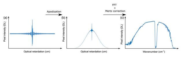
**Figure 2.** Summary of the processing algorithm from the interferogram to the IR spectrum. (a) Raw interferogram in one pixel of the camera. (b) Apodized interferogram. (c) IR spectrum in one pixel of the camera. FFT: fast Fourier transform; DL: digital level.
