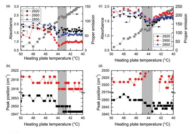
**Figure 8.** Effect of the sample temperature change on peak absorbance, peak position, and thermal emission in the left region depicted in Fig.7a. (a) Maximum peak absorbance and thermal emission and (b) peak position.
