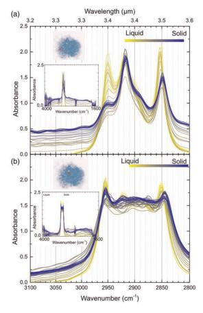
**Figure 7.** Paraffin absorbance spectra measured during the solidification for the two regions indicated in the image inserts (red square). (a) Left region and (b) central region. The inserted spectra show the entire range of measurement.
