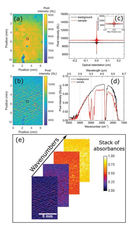
**Figure 4.** Data obtained before and after postprocessing of the interferograms. (a) Beam intensity of the background after the thermal emission removal. (b) Beam intensity after the thermal emission removal that passed through the polystyrene. (c) Interferograms of the black pixels in (a) and (b). (d) IR spectra obtained from the interferogram in (c). (e) Multispectral images of the sample absorbance obtained at the end of the postprocessing.
