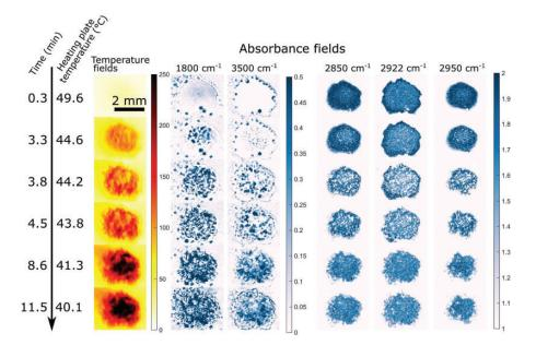
Figure 6. Temporal evolution of the paraffin multispectral absorbance and thermal fields. The relative temperature fields are in camera DL.
