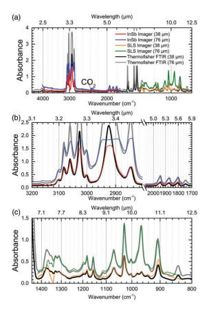
**Figure 5.** Comparison of the results between the FT-IR imager and a reference spectrum for the polystyrene samples. (a) Full spectra. (b) Focus in the  $3.1-5.9 \,\mu\text{m}$  range. (c) Zoom in the  $7.1-12.5 \,\mu\text{m}$  range.
