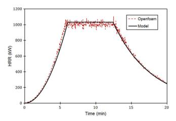
**Fig. 8.** Comparison between the modeled HRR prescribed as the boundary condition through the mass loss rate and the power released by the chemical reaction in the simulation.
