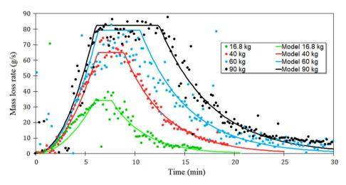
Fig. 7. Mass loss rates versus time for the four initial fuel masses. The model results (solid lines) are compared with the mass loss rate measurements (points).
