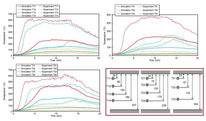
Fig. 13. Numerical and experimental temperatures for configuration 2. The distances are given in cm.
