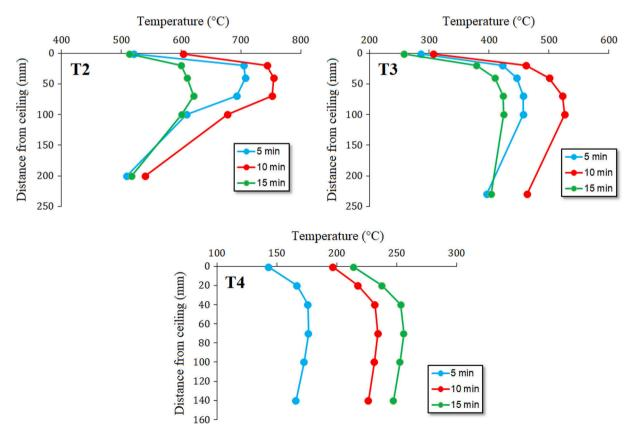
Fig. 9. Measured temperatures in the ceiling jet flow at trees T2, T3 and T4 five, ten and fifteen minutes after the ignition of the 90 kg hearth. The points stand for the locations of the sensors, which are also indicated in Fig. 4.
