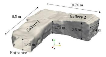
Fig. 1. Geometry of the quarry acquired by photogrammetry (P. Mora, Archéovision Production).
