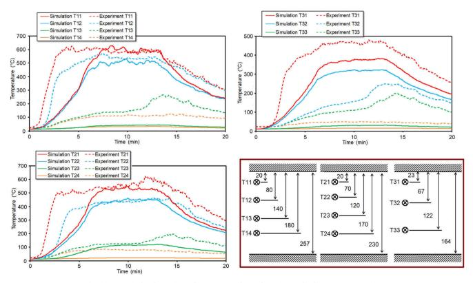
Fig. 14. Numerical and experimental temperatures for configuration 3. The distances are given in cm.
