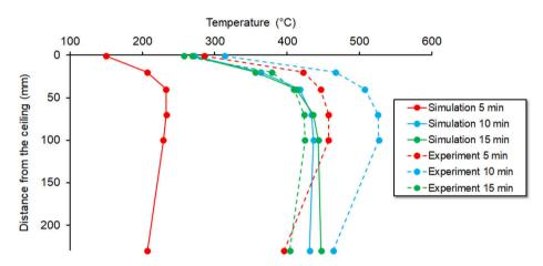
Fig. 11. Numerical and experimental temperature profiles near the ceiling at tree T3.
