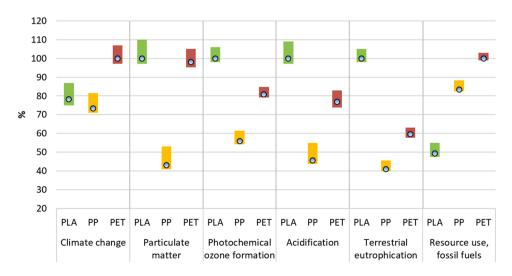
Fig. 8. Sensitivity analysis of electricity used for thermoforming per functional unit. The bars represent the ranges of variation of the environmental impact. The dots represent the baseline results. 100% values as Fig. 6 (the baseline value for the cups with the highest impact).
