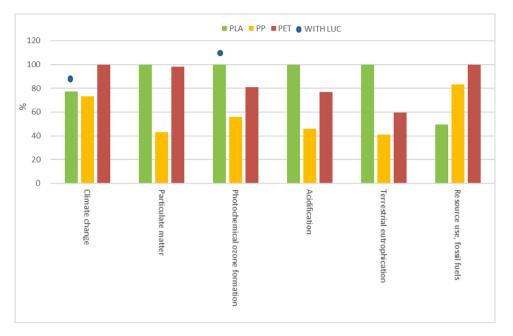
Fig. 6. Comparison of cradle-to-grave environmental impact 1000 single-use cups made from PLA, PP and PET (dots marking the impact of PLA with LUC).
