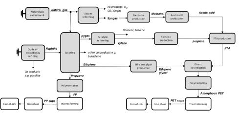
Fig. 2. Process flow diagram for petrochemical cups made of PP and PET produced in Europe. Gray boxes represent processes included in the PlasticsEurope's datasets for PP and PET. End of life: 30% recycling, 39% incineration and 31% landfilling.
