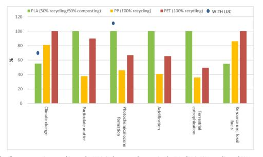
Fig. 9. Comparison of cradle-to-grave environmental impact for 1000 single-use cups by assuming the EoL of PLA: 50% recycling and 50% composting and the EoL of PP and PET: 100% recycling (highest impact as 100%). Dots marking the impact of PLA with LUC.
