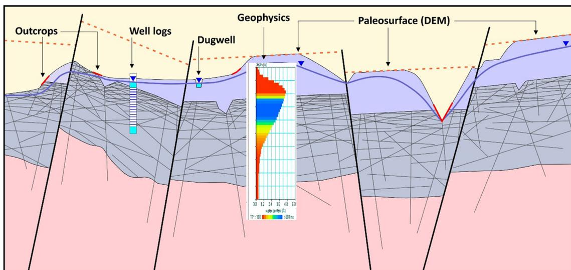
**Fig. 5** Methodology and data used for mapping HRA layers. See also the geological legend in Fig. 1. Note that the vertical scale is exaggerated, but that the relative thicknesses of the saprolite and SFL (1/3–2/3) are correct
