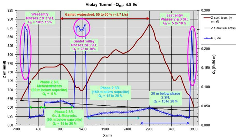
**Fig. 16** Violay (Loire Department, Massif Central, France) tunnel computed discharge  $Q_0$  (blue crosses - L/s/50 m of tunnel) according to the lithology, the weathering grade and the depth of the tunnel (black line) below the topographic surface (brown profile). The highest-discharge areas (purple circles) are located at both entries of the tunnel, and in the Gantet River Valley, where the tunnel crosscuts the SFL of the
