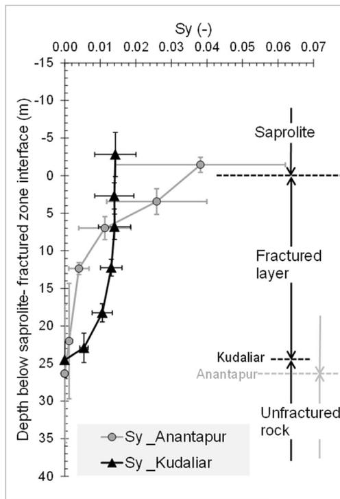
**Fig. 14** Average specific yield (Sy) in the weathering profile for the Anantapur and Kudaliar watersheds, Andhra Pradesh (now Telangana), India; bars depict standard deviations (from Dewandel et al. 2017b). With permission from Wiley
