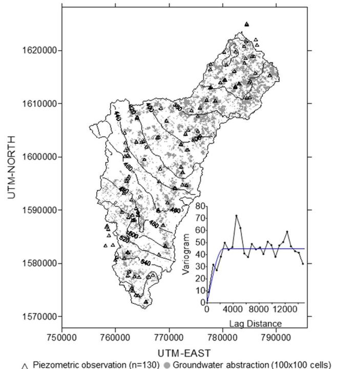
**Fig. 8** Piezometric map (in meters above sea level) on the 730-km<sup>2</sup> Anantapur watershed, Andhra Pradesh (now Telangana), India, and groundwater abstraction (on 100 m × 100 m cells; in grey); from Dewandel et al. (2017b). With permission from Wiley
