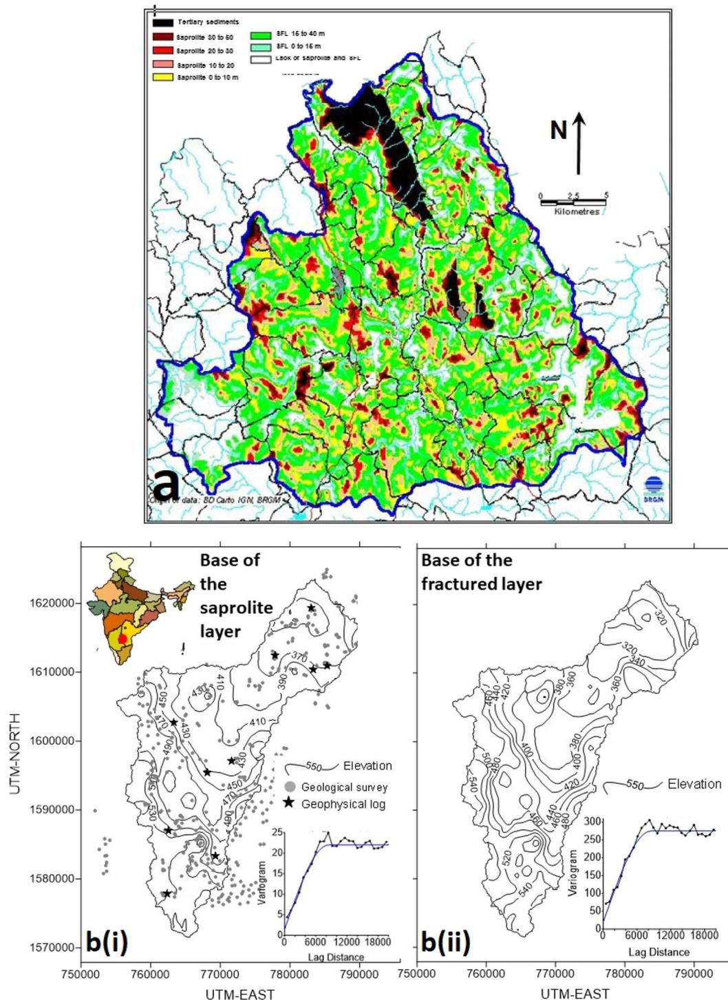
**Fig. 6** Examples of maps of the various layers forming hard-rock aquifers: **a** geological map of the weathering cover on the Truyère River, Lozère, France, watershed (700 km<sup>2</sup>): thickness of saprolite (increasing thickness from yellow, 0–10 m, to red and black, >50 m) and the fractured layer (increasing thickness from blue, 0–15 m, to green, 15–40 m), white: weathering profile totally eroded (Lachassagne
