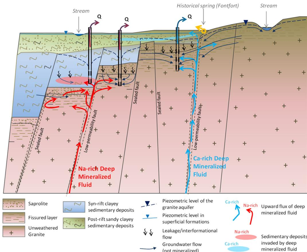
**Fig. 17** Conceptual model of a carbo-gaseous mineral hydrosystem (Saint-Galmier, Loire, France) where the fractured layer of the weathering profile constitutes the main aquifer (from Dewandel et al. 2017a). With permission from Elsevier
