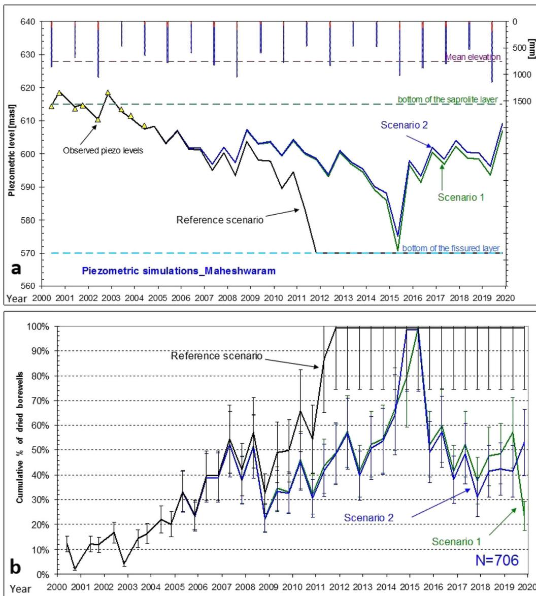
**Fig. 13** Example of long-term resource management simulation at the watershed scale, Maheshwaram, Andhra Pradesh (now Telangana), India: **a** mean piezometric level; **b** number of dried wells (Dewandel et al. 2010). With permission from Wiley
