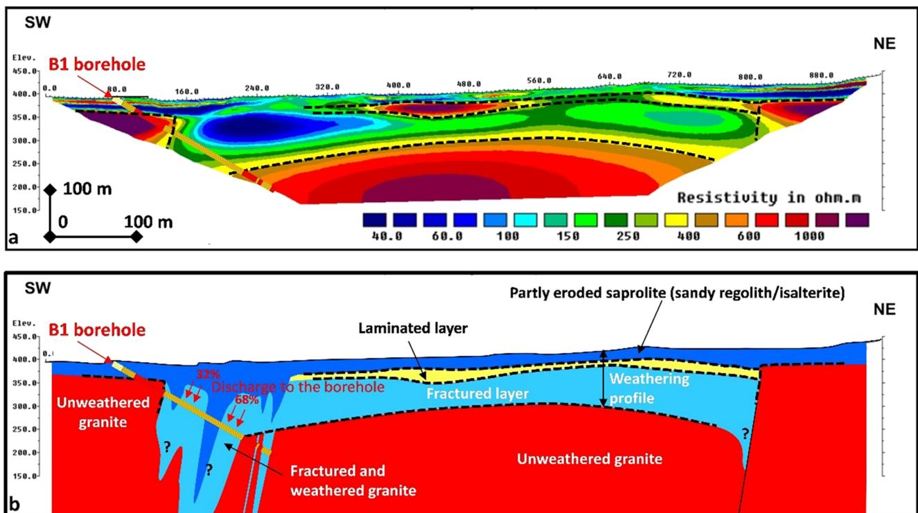
**Fig. 12** **a** Example of an electrical resistivity tomography geophysical profile in granitic weathered HR and **b** its hydrogeological interpretation. Saint-Galmier, Loire Department, Massif Central, France (from Belle
