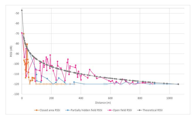
**FIGURE 4.** Signal reception quality as a function of the distance between the end-device and the gateway antenna for the three zones (closed area, partially hidden field, open field and theoretical RSSI).
