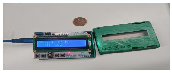
FIGURE 2. Hand held end-device (with its plastic shell) used to send data during the experiment.
