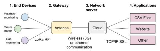
FIGURE 1. General architecture of the LoRaWAN network sensors (LPWAN-LoRa) tested in this study.
