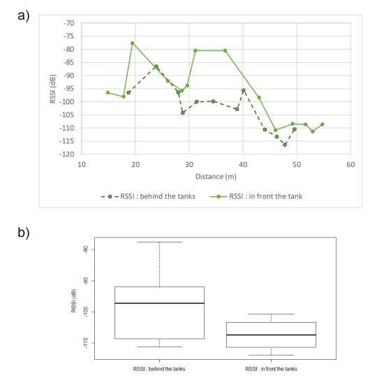
**FIGURE 7.** a) Signal reception quality as a function of the distance to the gateway antenna for end-devices behind or in front of the tanks, and b) comparison of RSSI variations with the sensor antenna outside and in the tanks by box plot.
