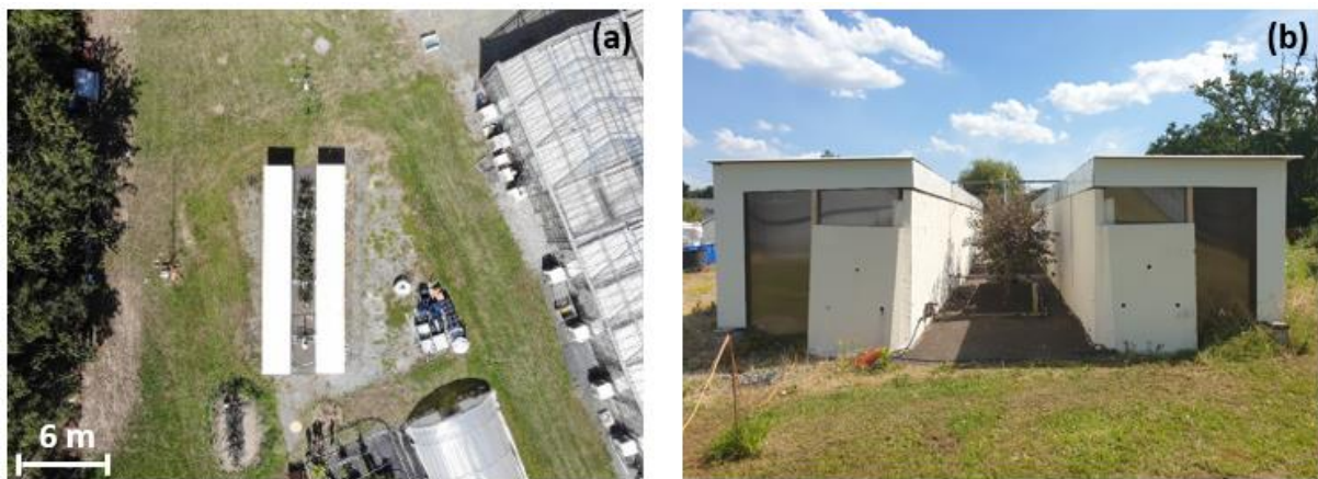
182 183 Figure 1 : Canyon street at 1/5 scale built at Institut Agro, in Angers (France). (a): top view, (b): front 184 view Photo credit: INRAE, OPAALE research unit.
