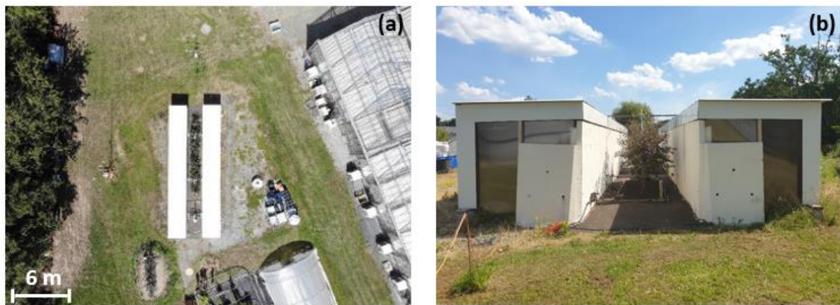
Figure 1 : Canyon street at 1/5 scale built at Institut Agro, in Angers (France). (a): top view, (b): front view Photo credit: INRAE, OPAALE research unit.
