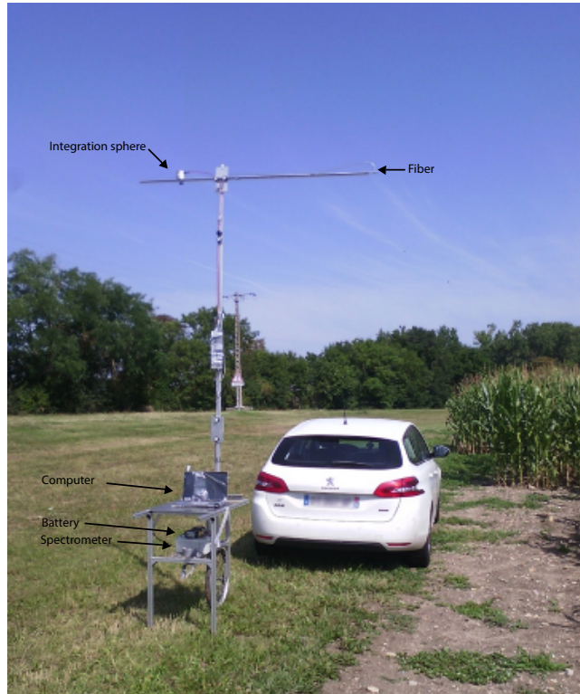
Figure 2: Image of the wheelbarrow embedding the spectral acquisition system, next to a car to visualize the height of the device.
