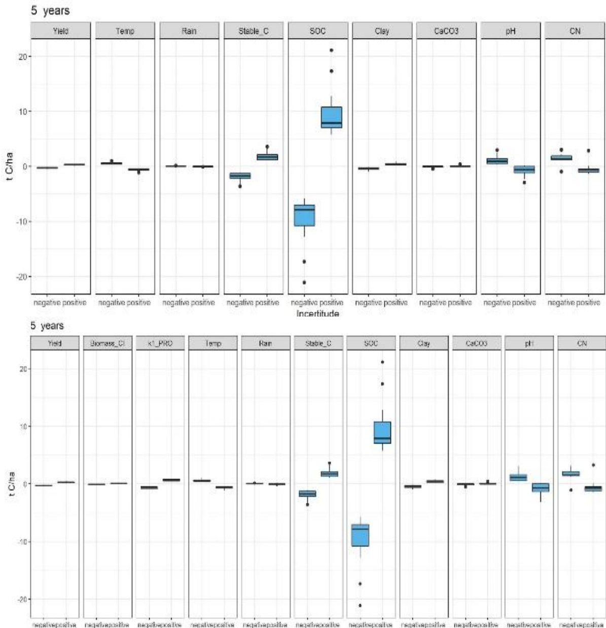
Figure 1. Sensitivity analysis of the final soil C stock after 5 years for 2 practice scenarios: without (top) and with (bottom) intermediate crops and PROs (residual organic products) applications. Influence of the relative uncertainties (negative bound, positive bound) of the input variables and parameters of the AMGv2 model on the C stock. Each box shows the variability of the results for the 12 sites analyzed. The final stock is highly dependent on the initial stock (high sensitivity to the SOC variable).
