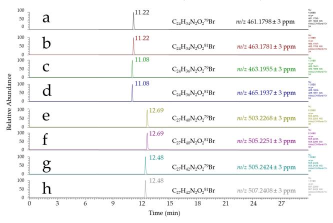
**Figure 2.** LC–HRMS-extracted chromatograms: (**a**,**b**) ion chromatograms of the <sup>79</sup>Br and <sup>81</sup>Br isotopomers of HHE-APEBA; (**e**,**f**) ion chromatograms of the <sup>79</sup>Br and <sup>81</sup>Br isotopomers of HNE-APEBA; and (**c**,**d**,**g**,**h**) ion chromatograms of their corresponding reduction byproducts.
