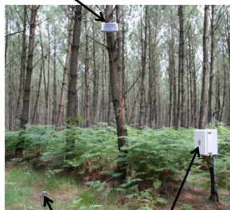
Well to measure water table depth with a TDR sensor
