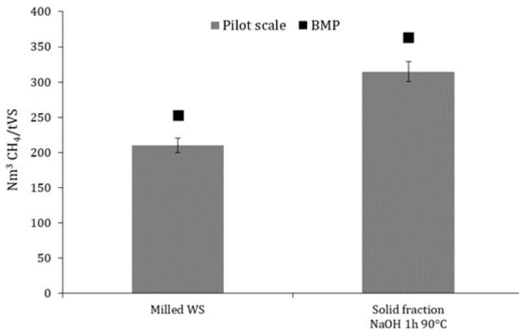
Figure 7. Comparison of methane potential (BMP vs. pilot-scale).
