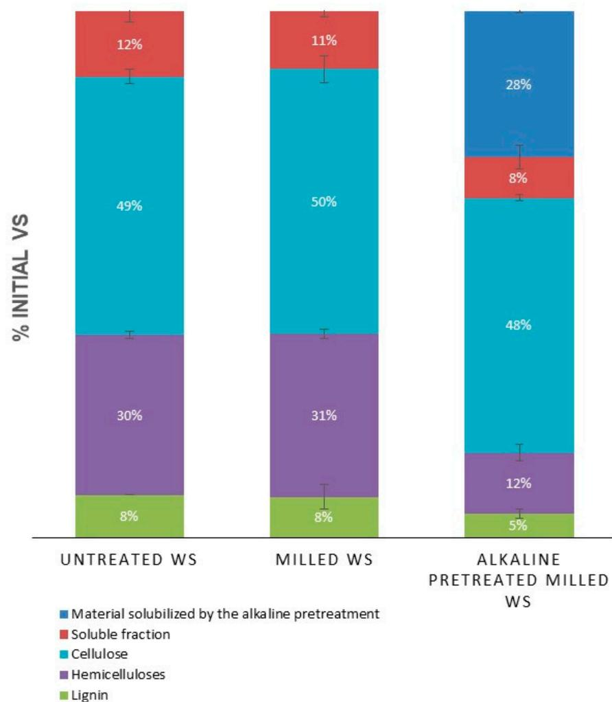
**Figure 2.** Chemical composition determined by Van Soest fractionation for untreated WS, milled WS, and alkaline-pretreated milled WS, expressed in terms of % initial VS. Values correspond to mean  $\pm$  standard deviation of measurement performed in duplicate.
