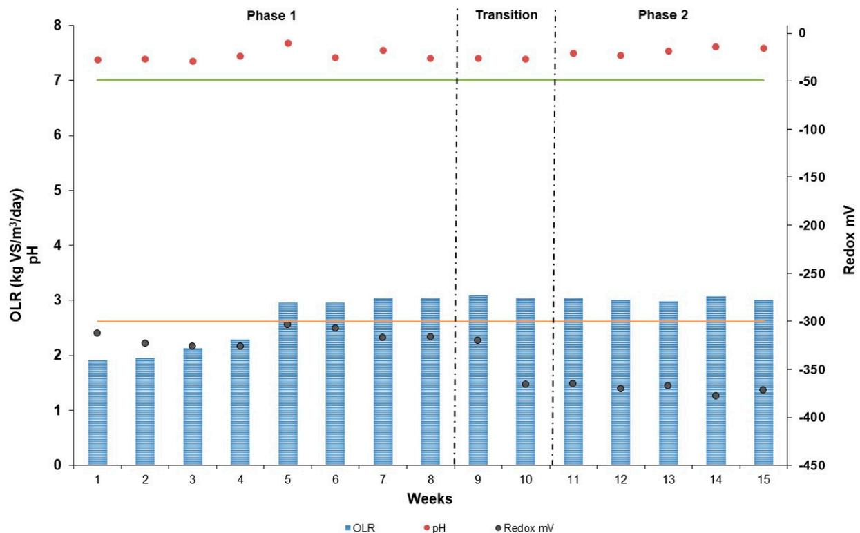
**Figure 4.** Organic loading rate (OLR), pH, and potential redox of the pilot scale reactor during the various running phases.
