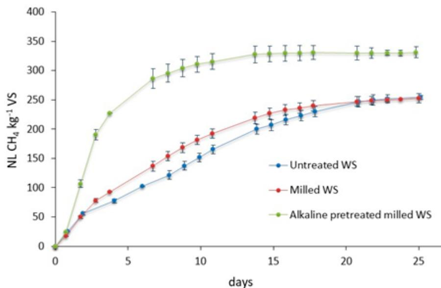
**Figure 3.** Cumulative methane production (NL CH<sub>4</sub> kg<sup>-1</sup> VS) during BMP tests of untreated WS, milled WS, and alkaline-pretreated milled WS.
