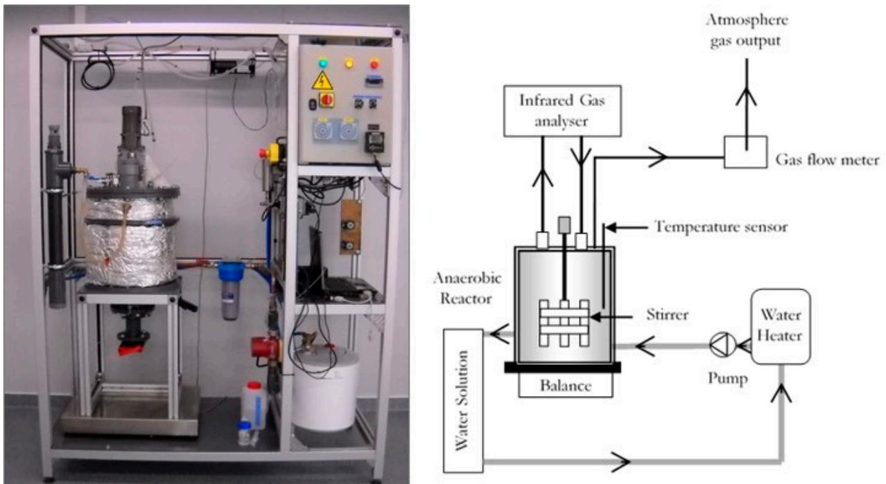
**Figure 1.** Schematic view of the anaerobic digester pilot.
