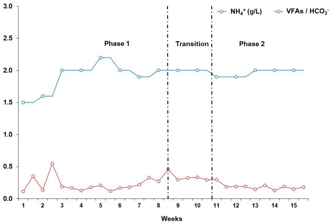
Figure 6. Ammonium (NH<sub>4</sub><sup>+</sup>) content and VFAs/HCO<sub>3</sub><sup>-</sup> ratio during the different phases of the continuous pilot assay.
