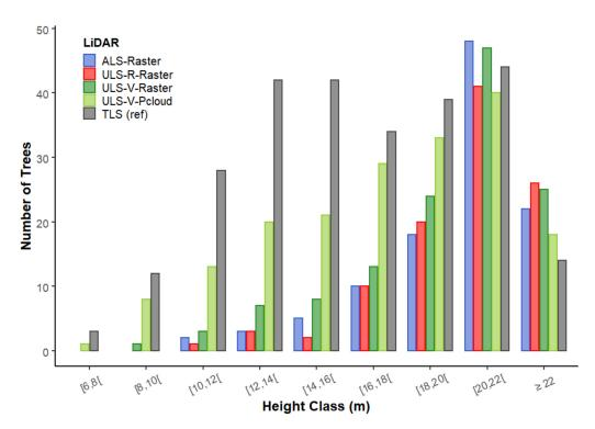
**Figure 12.** The distribution of trees, by height class, detected from ALS-Raster (leaf-on), ULS-R-Raster (leaf-on), ULS-V-Raster (leaf-off), and ULS-V-Pcloud (leaf-off) that were matched with a TLS reference tree (Ntrees<sub>paired</sub>).
