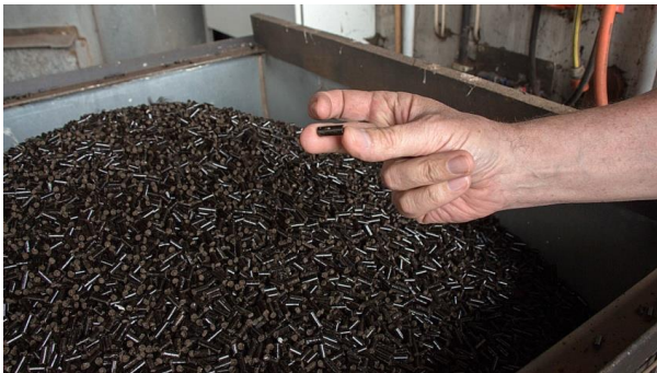
Figure 20: Pellets from Digestate (picture credits: IBBK Fachgruppe Bigoas GmbH)
