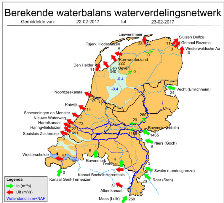
Figure 1 Example display of the operational water management system for the Netherlands, showing a daily computed or forecasted water balance for the surface water network for the Netherlands.
