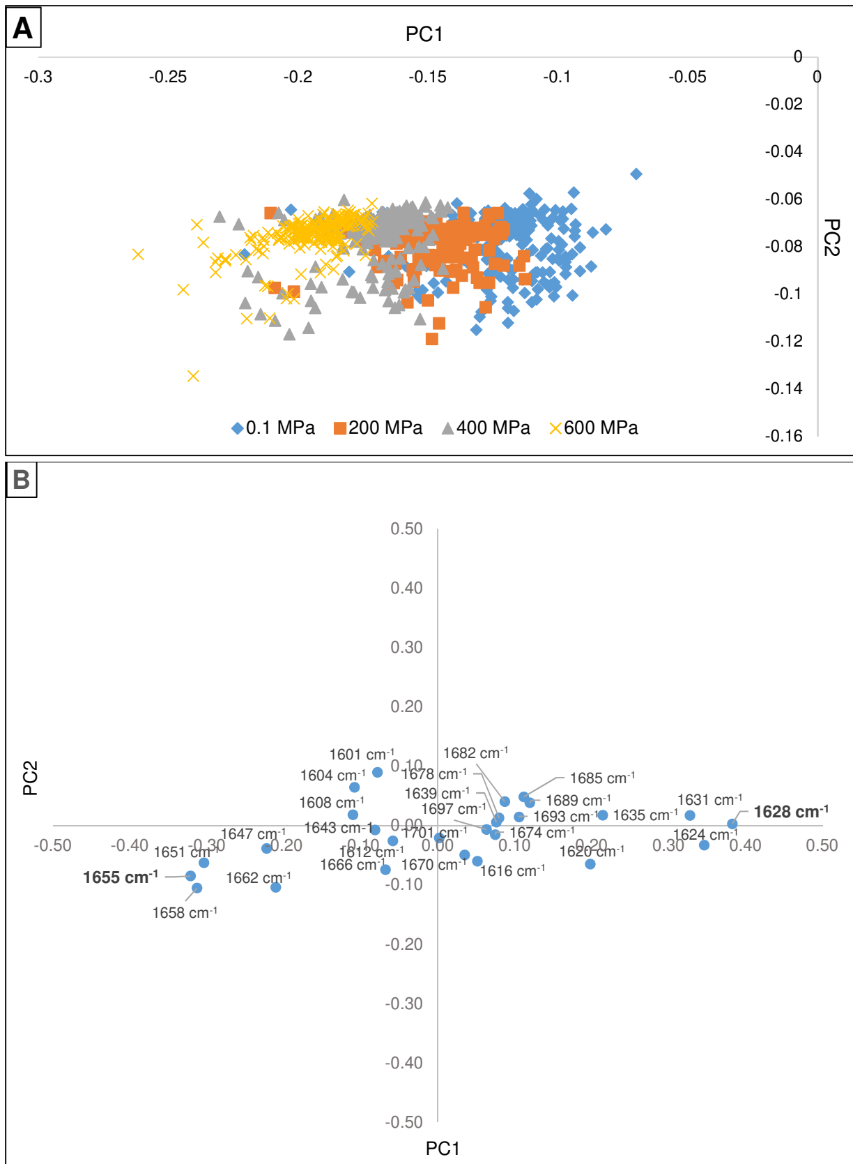
Figure 5: Principal component analysis (PCA) of the second derivative of the amide I (1600-1700 cm -1 ) band (A). Pressure groups are separated along the first principal component (PC1).
